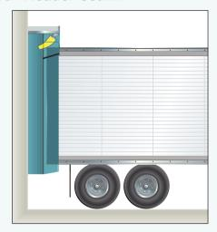
When vehicle is in position at the dock, the helical torsion springs of the pivoting head member provides consistent tension force over the width of the unit while ensuring the foam head member conforms to the top of the trailer creating a water-tight wiper seal.
